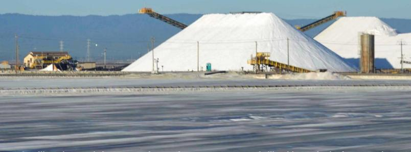
Cargill produces salt for water softeners from evaporator ponds like this one in the foreground at the southern end of San Francisco Bay.
